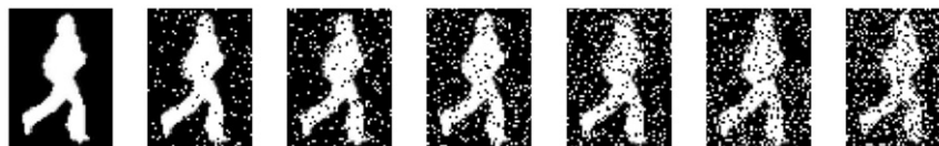
Fig. 19. From left to right are the noise-corrupted silhouettes with different degrees of synthetic noise, which are 0, 0.1, 0.15, 0.2, 0.25, 0.3 and 0.35, respectively.
