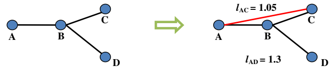
Fig. 5. An example of linearity measurement indicates that the data point C which is not the neighbor of A but its linearity is strong enough will add an edge between them. However, the data point D which is not the neighbor of A and the linearity is not strong enough will not add an edge between them.
